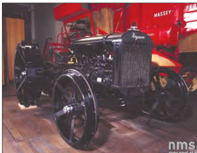
The "Black Tractor" was Ferguson's first prototype, built in 1933 to test his "Ferguson System" three-point linkage/draft control concepts. It proved to be less than satisfactory.
